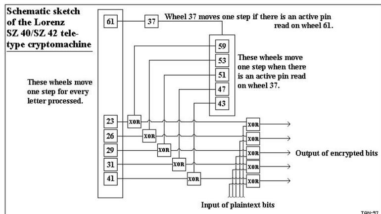
Figure 2: SZ-40 Wiring diagram
