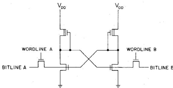
Fig. 9. Dual-port static register cell.
