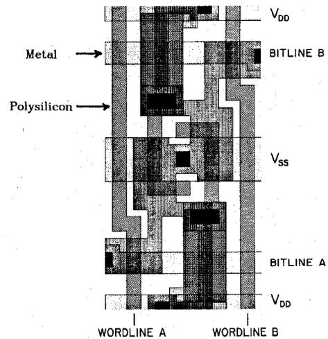
Fig. 10. Layout of dual-port static bit cell.
