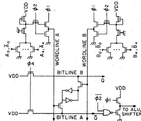
Fig. 11. Register file cell with decoders and single-ended sensing logic.
