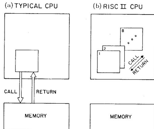
Fig. 3. Procedure call and return in register-based machines.
