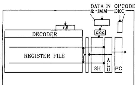
Fig. 1. Allocation of chip area resources in RISC II.
