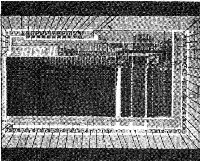
Fig. 8. RISC II chip photomicrograph.
