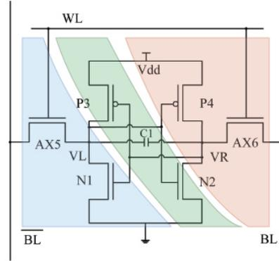
Fig. 3. Capacitor based SRAM Design
