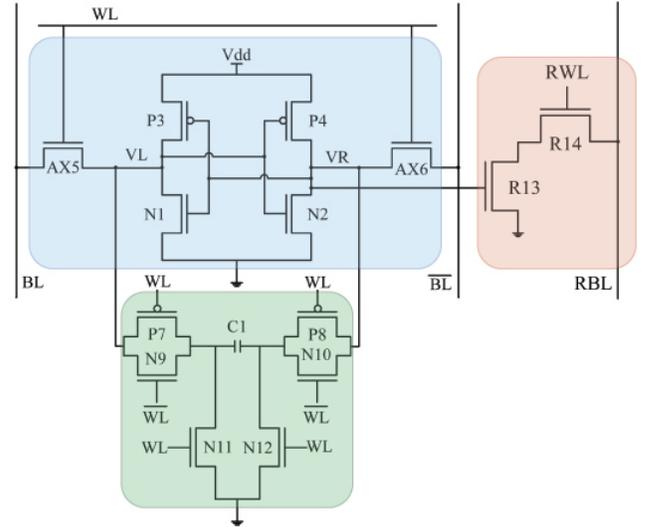
Fig. 5. SRAM-SCS design with full component separation
