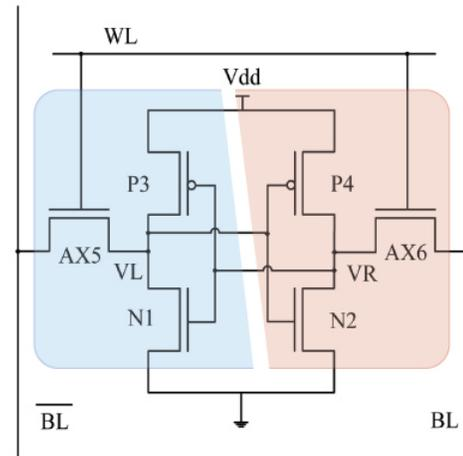
Fig. 1. Classical 6 Transistor SRAM Design
