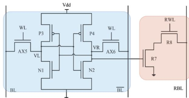
Fig. 2. 8 Transistor SRAM Design
