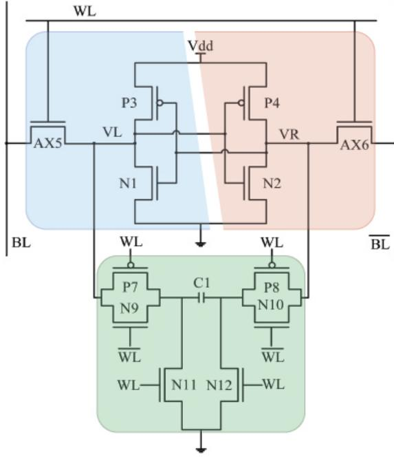
Fig. 4. SRAM-TCT design with separated protection circuit
